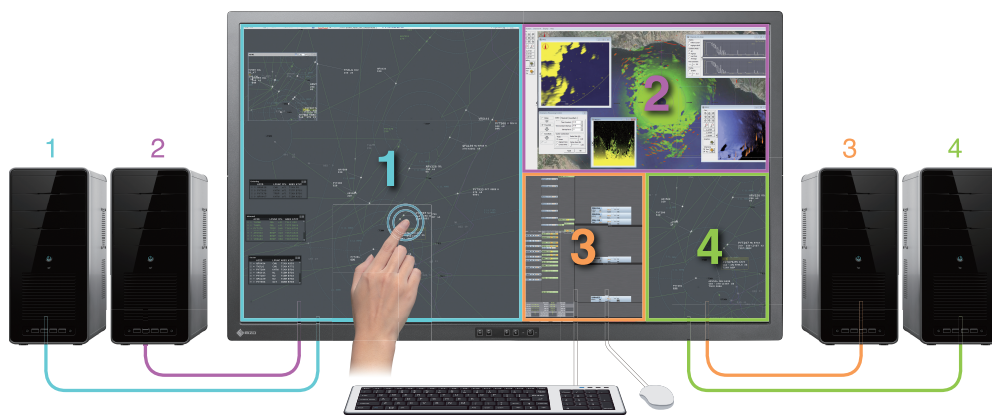
Above: EIZO's monitors with IDP and SwitchLink allow operators to display up to four video sources simultaneously and automatically switch between them using a single mouse and keyboard
