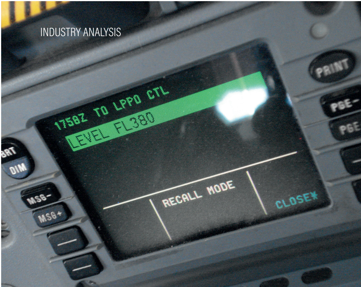
Left: A Datalink Control and Display Unit, the pilot interface for CPDLC text messages
