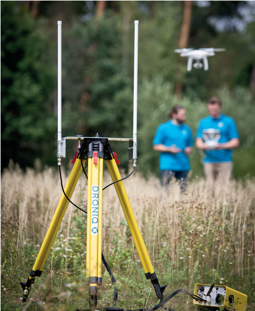
Left: The ground based situational awareness system (GBSAS) receives the position data for example of other aircraft in the surrounding airspace (Image: Droniq)
