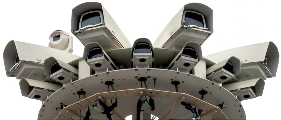
Above: The IRTOS 4K video camera system, which produces data that can enhance ATC system performance
